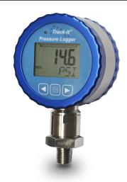
the event of a power loss. *Track-It*™ Pressure Transmitter/Data Loggers can be ordered in various ranges (see back for details). The logger is packaged in a rugged anodized aluminum and stainless steel housing and has a standard 1/4″ NPT fitting (1/2″ NPT for 8700 and 14,500 ranges).
