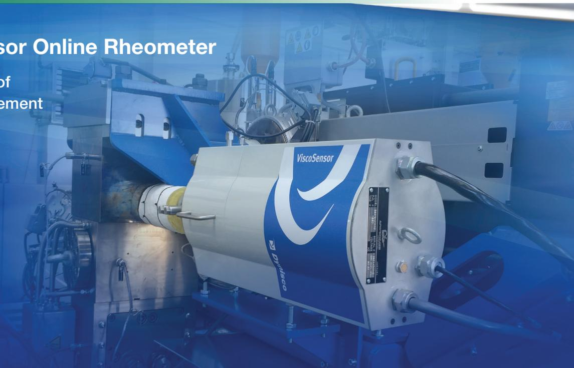
A capillary viscometer forces material through a small diameter capillary die creating a pressure drop across the die. By controlling the material's shear rate through the die or shear stress across the die, apparent viscosity or melt flow index is obtained. The ViscoSensor uses differential pressure across the capillary die for either a control point for melt flow index measurement or as a measurement point for apparent viscosity calculations.
