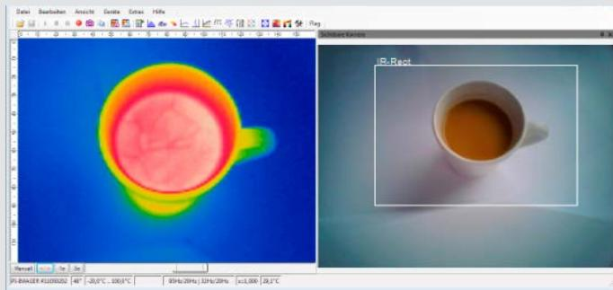
The software can be used to save the recording from the thermal imaging camera as video sequences which can then be saved for analysis later on. The video sequence is recorded for every pixel including all temperature information. An integrated screen capture function makes it simple to retrospectively generate videos in wmv format.
