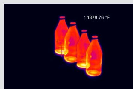
Hot-spot measurement in the production of glass bottles.
