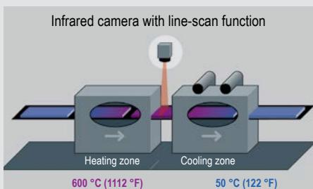
Construction of a glass tempering plant.
