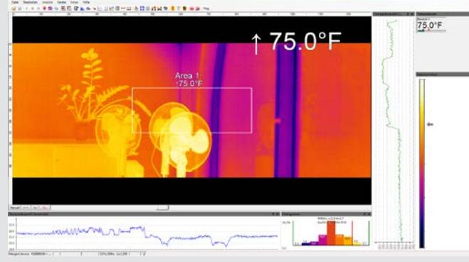
The PIX Connect software gives you the option of grouping together several cameras within a software instance, i.e. the field of view of several infrared cameras are merged together to make a single picture. For processes with several control points in particular, it is helpful to concentrate the various angles on one screen. Merging several cameras also makes it possible to get an all-round view of a 3D object.
