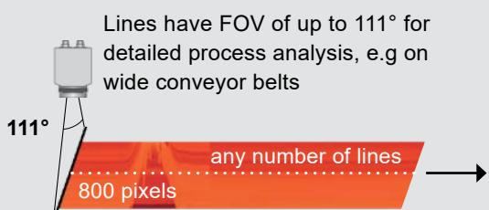
Up to 32 Hz data recording\* of unlimited lines which in turn produce a thermal image of any given resolution
