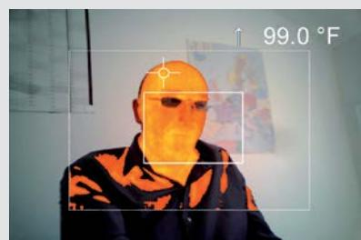
Cross fade of a VIS image above 35 °C (95 °F)
