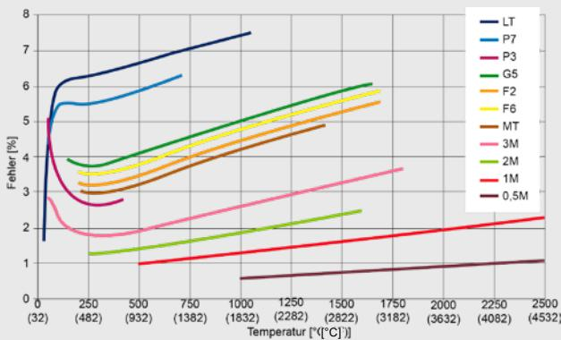
*Short wavelengths reduce measurement errors on surfaces with low, unknown or changing emissivity. This occurs mostly with metals. The diagram above shows the measurement errors across different wavelengths if the emissivity is wrongly adjusted by only 10 percent.*
