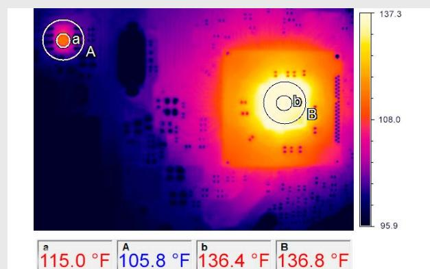
IR image of an electronics circuit board – adaptation of the measurement spot to the object size
