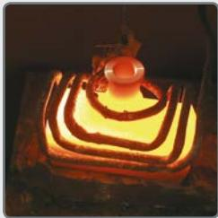
Induction heating has acquired high importance within the area of heat treatment of metal. The aimed-for texture structure of the metal depends on the ideal temperature time process.
