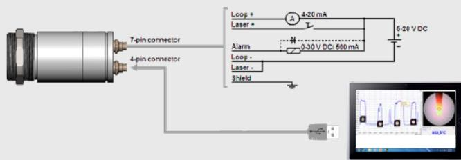
Analog operation mode: 4–20 mA and alarm interface. Setup & installation via USB cable (hot Plug & Play)
