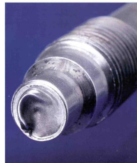
Transducer damage caused by mis-machined hole.
